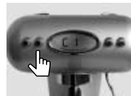
Start the extraction of the coffee while holding in button (3) until the desired amount of coffee is in the cup, than release the button. After preparation, the machine will save the respective time duration. You can also change the C2 time using the same procedure.
